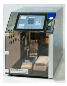
Accurate contact and non-contact sample preparation system for handling of chemical or biological solutions or suspensions
